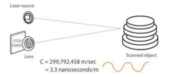
Laser phase-shift systems are another type of time-of-flight 3D scanner technology, and conceptually work similarly to pulse-based systems. In addition to pulsing the laser, these systems also modulate the power of the laser beam, and the scanner compares the phase of the laser being sent out and then returned to the sensor. For reasons that are beyond this web page's scope, phase shift measurement is more precise.
